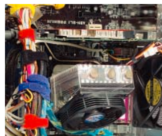
The Vapochill is quieter than the recommended standard AMD cooler
